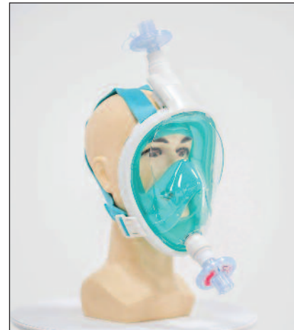
The CanCov medical mask was partially invented by Uxbridge entrepreneur Adam Ruppel. The mask is a fully sealed dual filtered mask created to assist medical staff during the COVID-19 pandemic.
